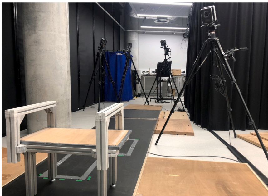
Fig. 1. Typical gait laboratory showing 4 motion capture cameras, 2 ground force plates and an instrumented chair.
